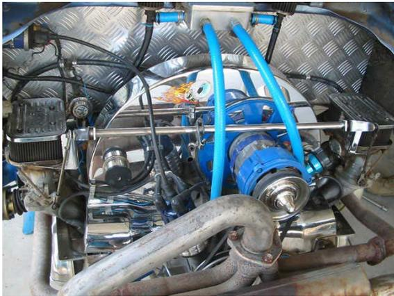
The engine is fed by twin 44IDF webbers, with the scat air cleaners converted to a bolt-on design to ensure no sand finds it's way into the engine. I usually run the engine on 98 octane PULP which is ignited by a 009 mechanical dizzy running electronic points. Vacuum dizzy's cause high performance engines to knock while offroading at low rpm. The exhaust gases are fed out through thunderbird 4-1 extractors into a SS genie turbo muffler and 3x4" oval exhaust tip.
